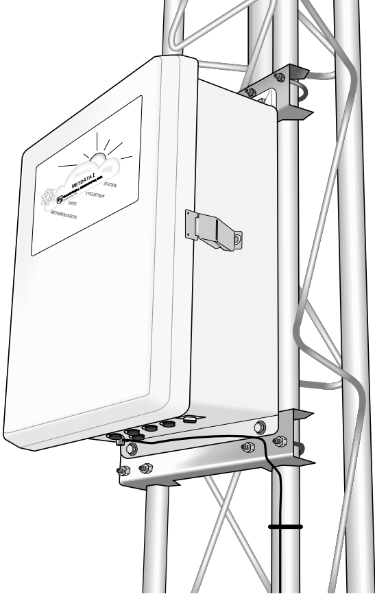
FIGURE 3.1-2. MetData1 Enclosure on UT10 or UT30 Tower
