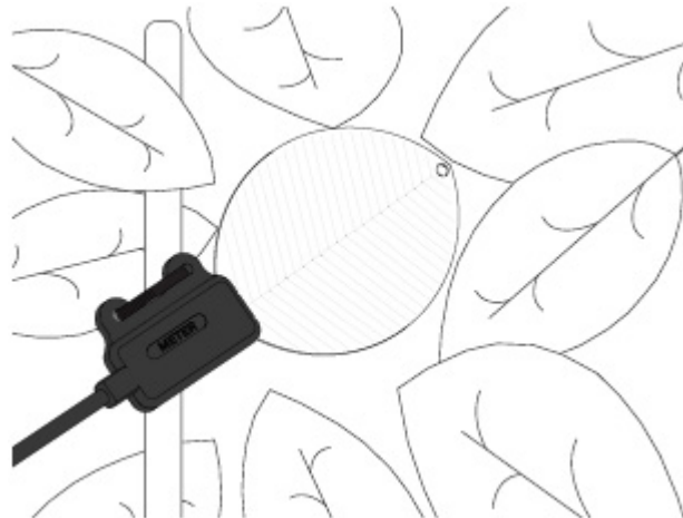
FIGURE 7-2. Top view of a typical LWS installation
