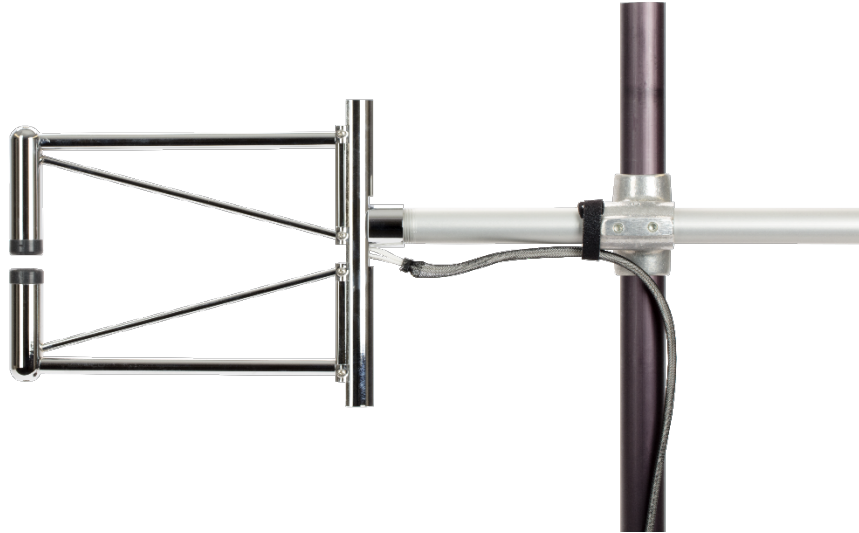
FIGURE 6-1. Mounting KH20 to a tripod
