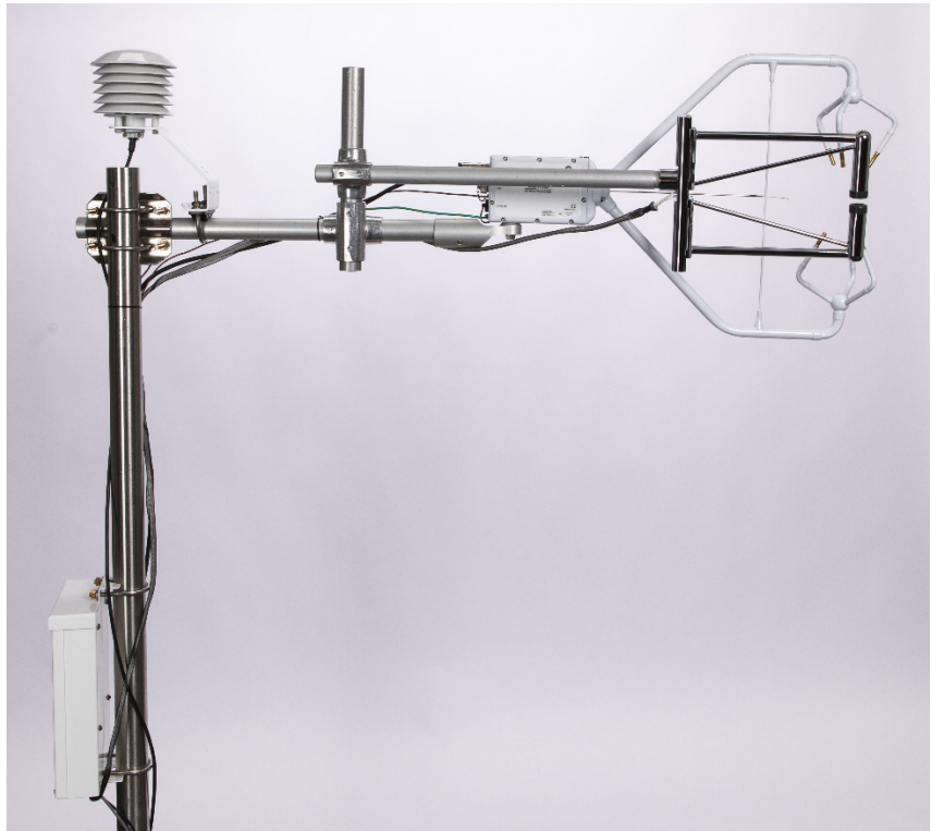
FIGURE 6-4. KH20, CSAT3B, and electronic box mounted on a mast
