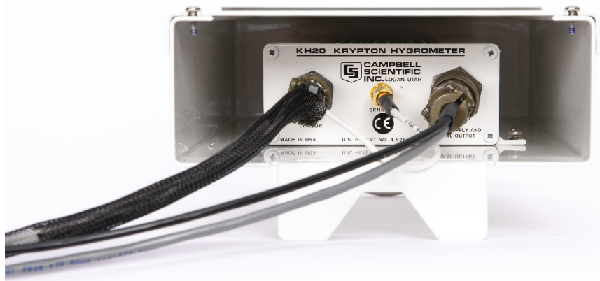
FIGURE 6-2. Attaching cables to the electronics box
