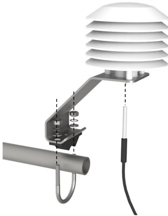
FIGURE 6-4. Mounting the IRGASON temperature probe
