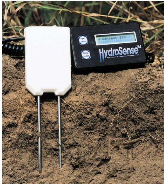
FIGURE 1-1. The HydroSense system consists of the CS620 sensor (left), the CD620 display (right), and two rods.
