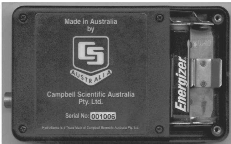
FIGURE 8-1. Rear view of the HydroSense display unit with battery cover removed
