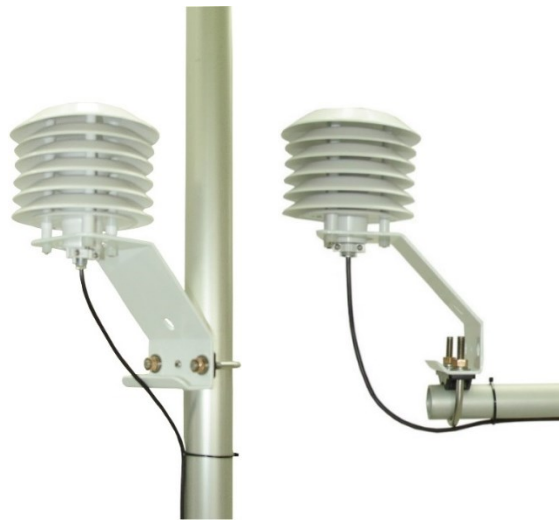
FIGURE 7-3. HMP60 and 41303-5A Radiation Shield on a tripod mast (left) and on a CM202 Crossarm (right)
