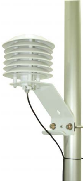
FIGURE 2. HMP50 and 41303-5A Radiation Shield on a Tripod Mast
