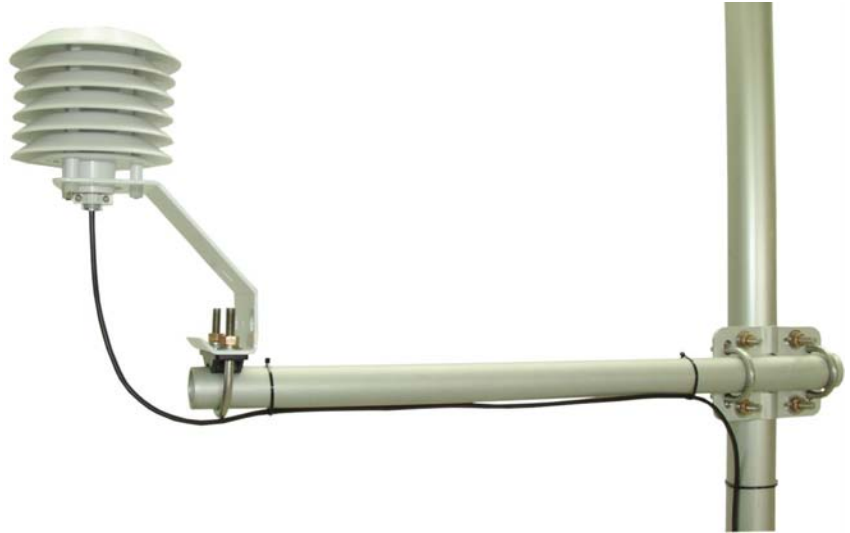
FIGURE 3. HMP50 and 41303-5A Radiation Shield on a CM202 Crossarm
