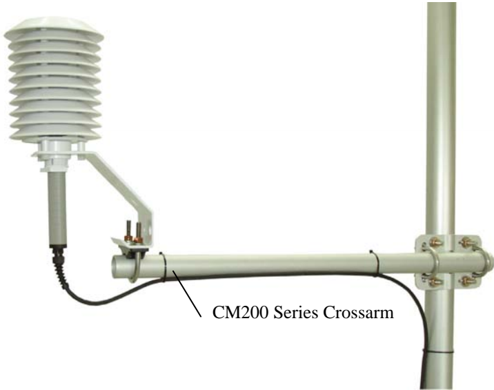
FIGURE 3-2. HMP45C and 41003-5 Radiation Shield on a CM200 Series Crossarm
