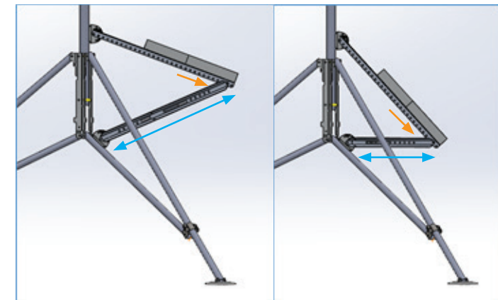
Figure 9: 20 degree to 50 degree mounting angles.
