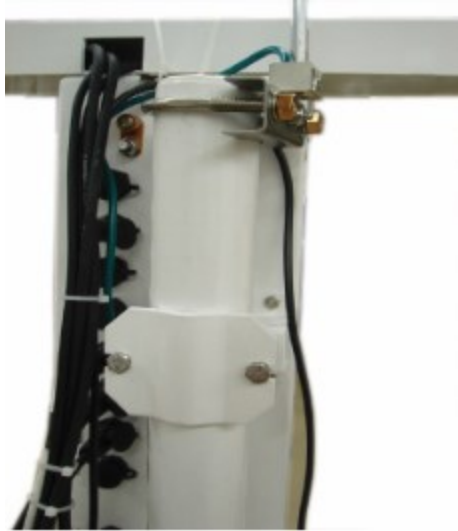
FIGURE 6-29. Loosely drape antenna cable over back of enclosure
