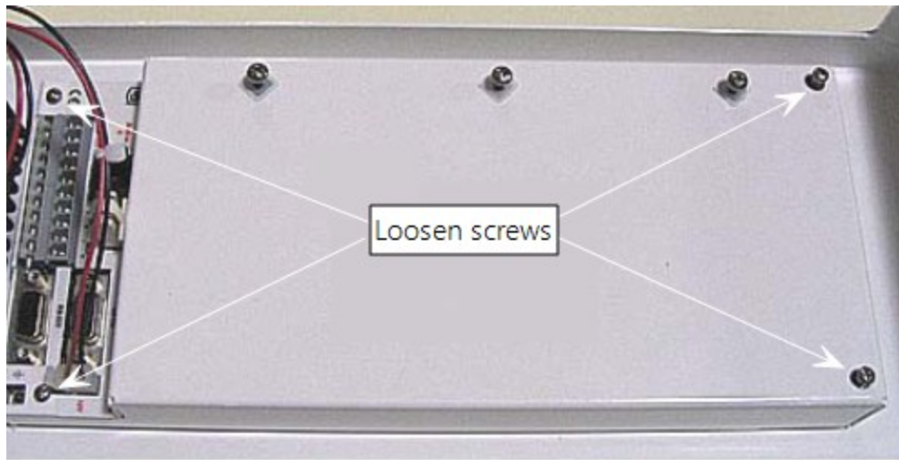
FIGURE 6-13. Screws that secure the electronics cover
