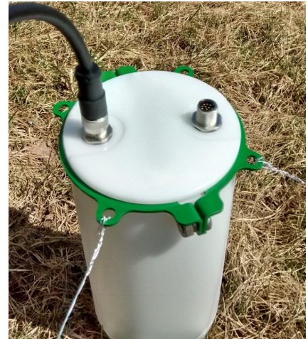
Figure 5 An eosFD deployed in the field, with uncovered aux port
