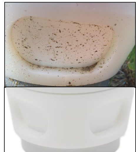
Figure 6 Top: Mildly fouled membrane. Bottom: Clean eosFD membranes
