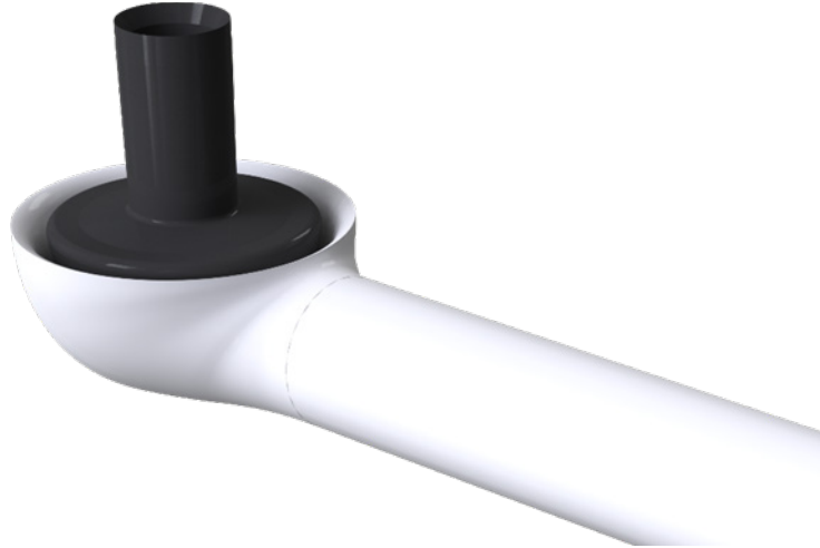
FIGURE 9-5. The underside of the intake of the older design sample cell showing the inline filter with rain diverter in black
