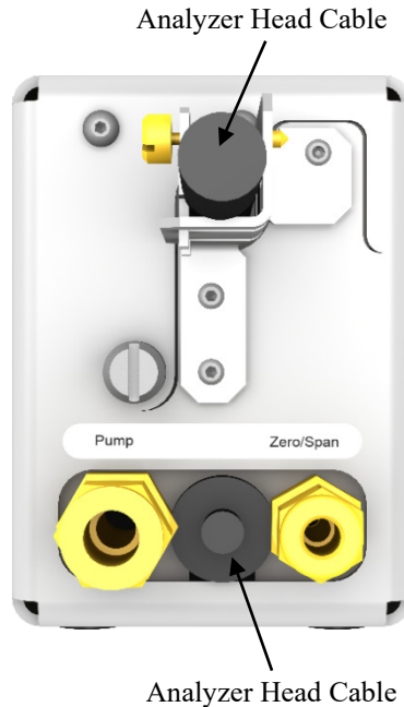
FIGURE 6-10. End view of EC155 analyzer showing ports for pump outlet (vortex bypass tubing and filter assembly not shown) and zero-and-span intake
