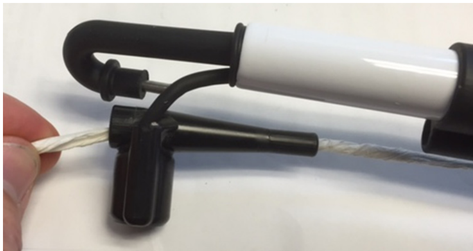
FIGURE 9-4. A damp paper towel or cloth used to floss and clean inside surfaces of vortex chamber
