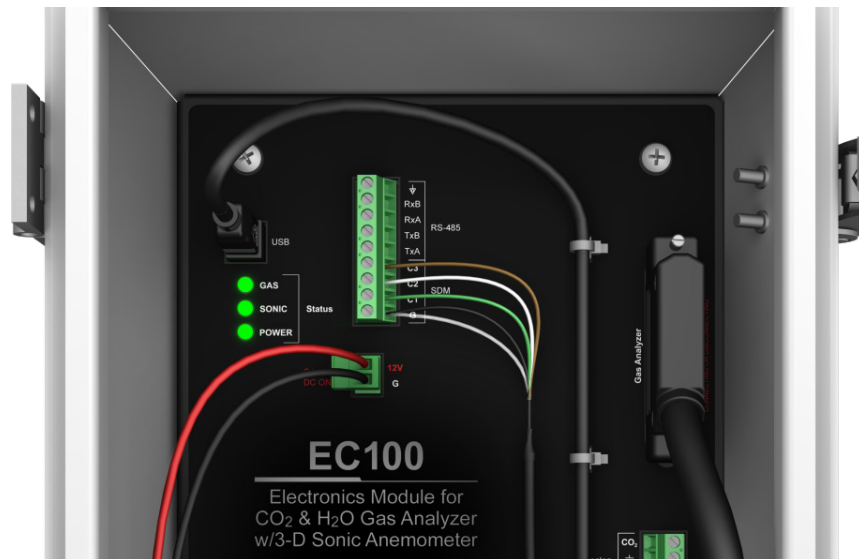
FIGURE 8-3. LED status during normal operation
