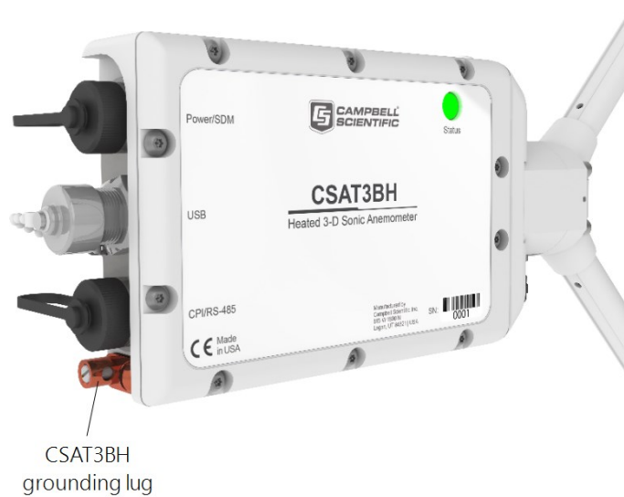
FIGURE 6-11. Grounding lug of CSAT3BH
