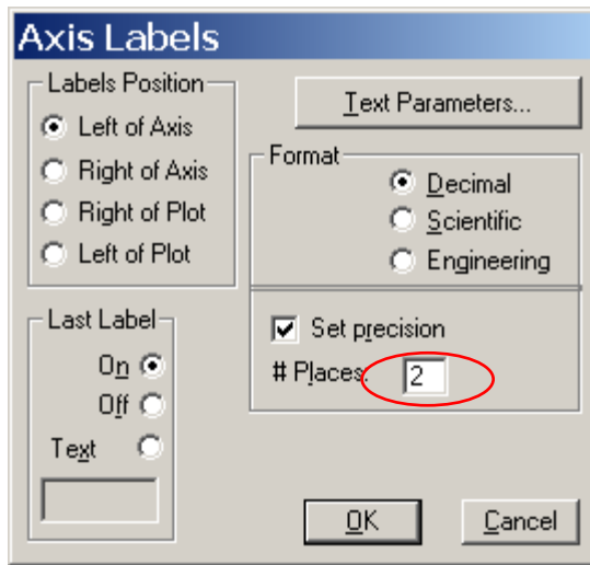
FIGURE 11-5. Recommended settings for the wind vertical axis labels
