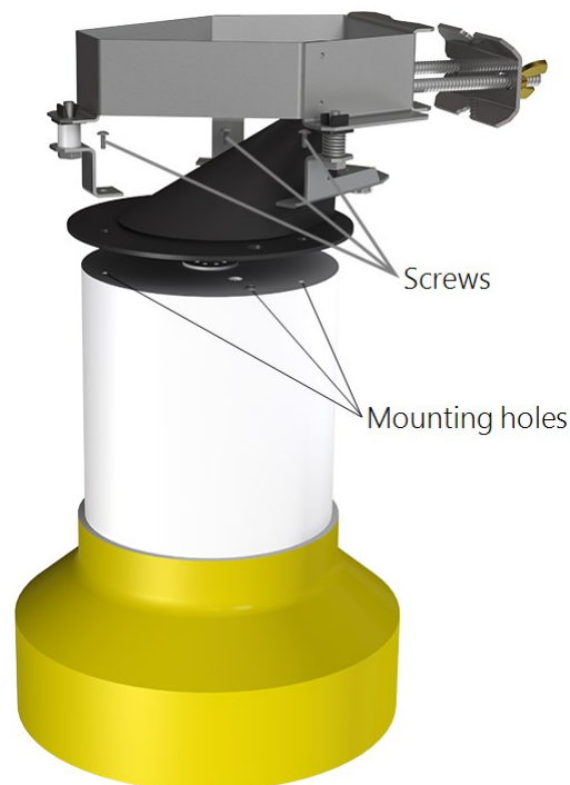
FIGURE 6-6. Mounting CM270 to the rain gage
