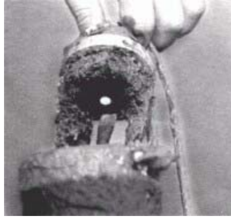
FIGURE 5-1. Preventing Bio-fouling of the CS510-L
