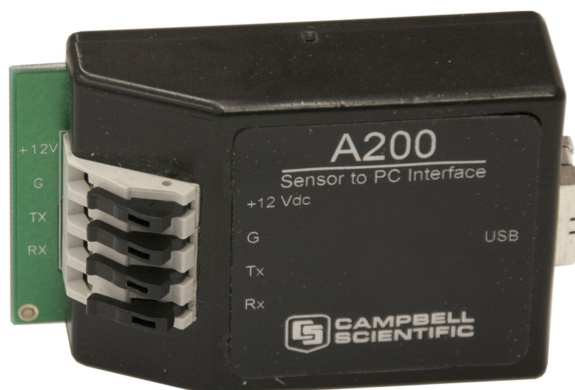
FIGURE 8-1. A200 Sensor-to-Computer Interface
