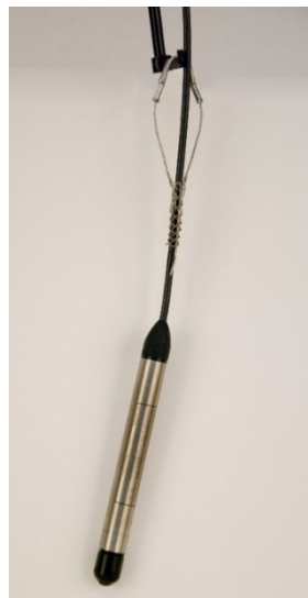
FIGURE 7-1. Transducer suspended with split mesh cable grip
