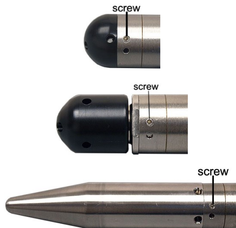
FIGURE 7-4. Screws on the standard nose cone (top), NPT nose cone (middle), and weighted nose cone (bottom)
