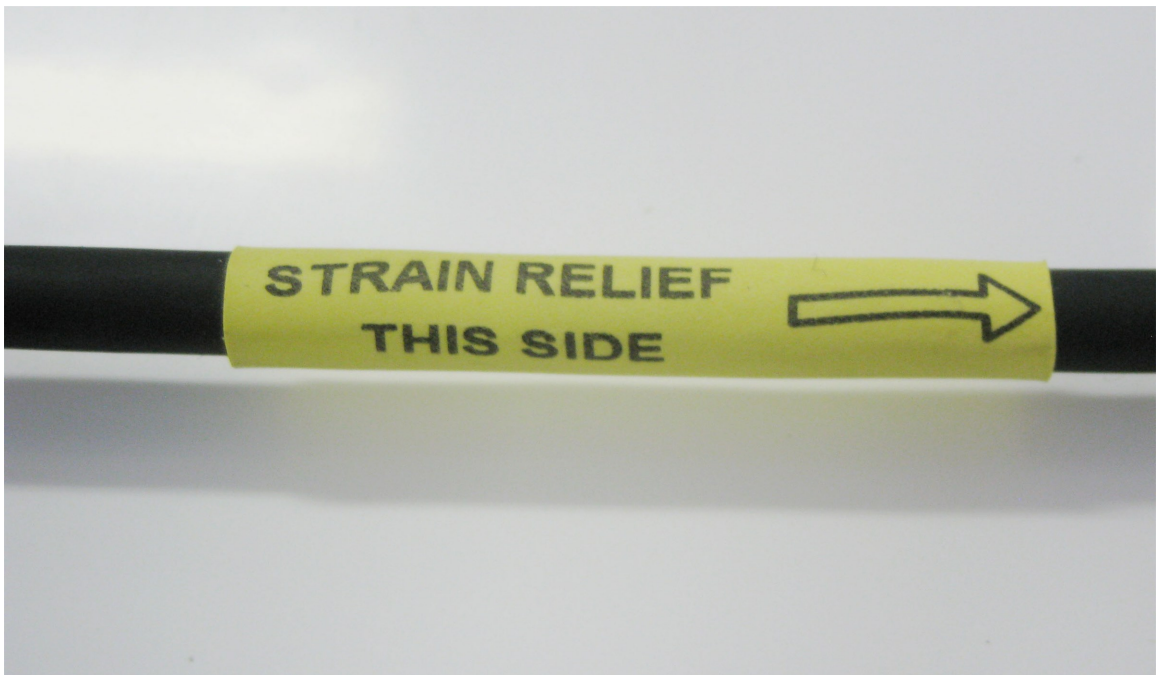
FIGURE 7-3. Strain relief label on the cable
