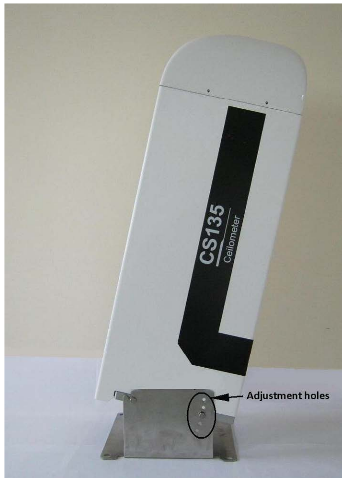
Fig 4.2 Setting the Tilt Angle
