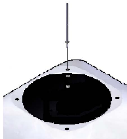
Fig 4.11 Attaching Bird Spikes to the CS135 cowl
