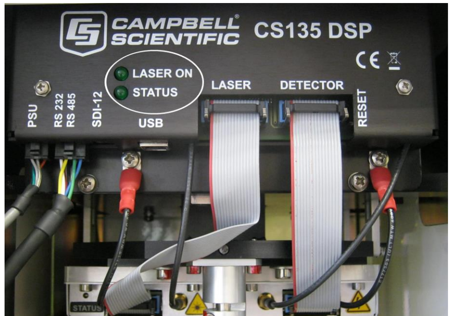
Fig 7.3 Diagnostic LED indicators
