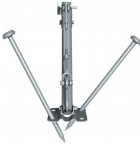
FIGURE B-2. Staking the tripod feet
