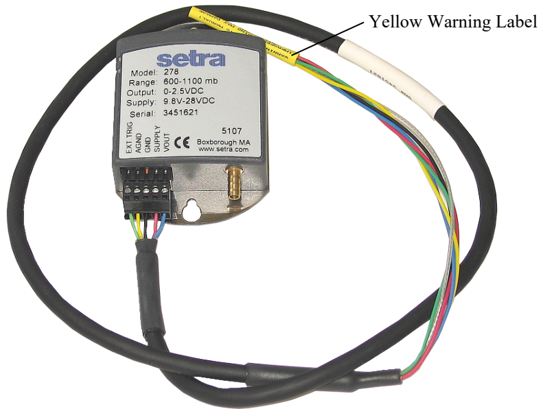
FIGURE 7-3. CS100 and cable with warning label
