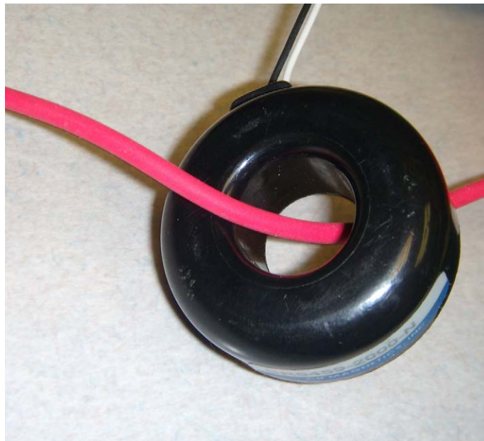
FIGURE 2. AC load wire installed in CS10 (color of ac load wire can vary)
