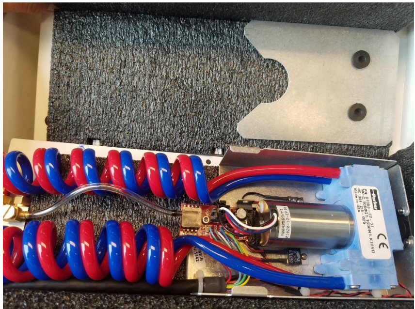
FIGURE H-13. Proper positioning of CPEC300 in shell cover
