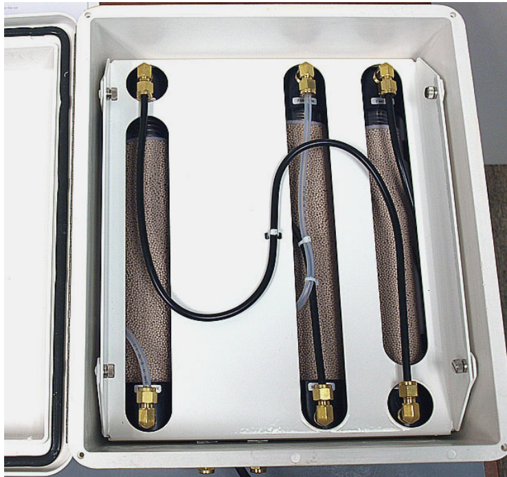
FIGURE G-2. CPEC310 scrub module interior
