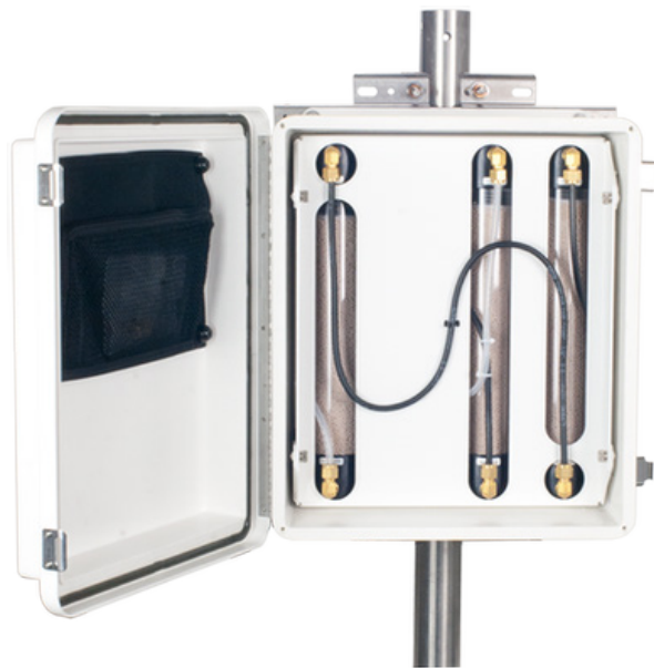
FIGURE 4-18. CPEC310 scrub module (shown with enclosure lid open)
