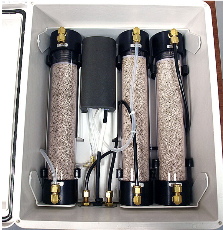
FIGURE G-3. Interior of CPEC310 scrub module with tubing and cover removed
