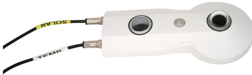
FIGURE 7-3. The CNR4 sensor with SOLAR and TEMP cables
