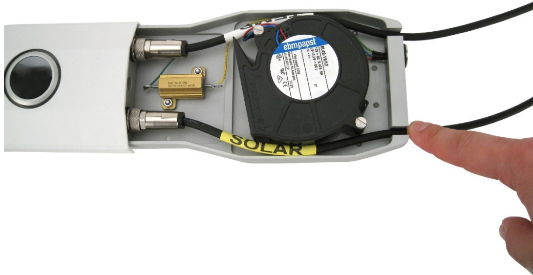
FIGURE C-3. Making sure the cables are clear from the edges
