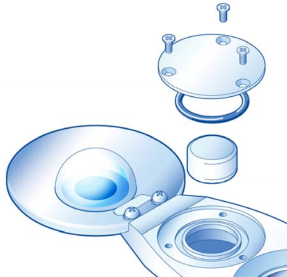
FIGURE 8-3. Replacing Drying Cartridge (first replacement cartridge comes with the CNR2)
