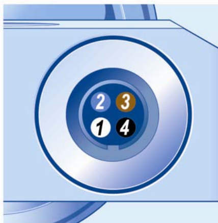
FIGURE 5-1. Pin Layout on Campbell Scientific Black Cable
