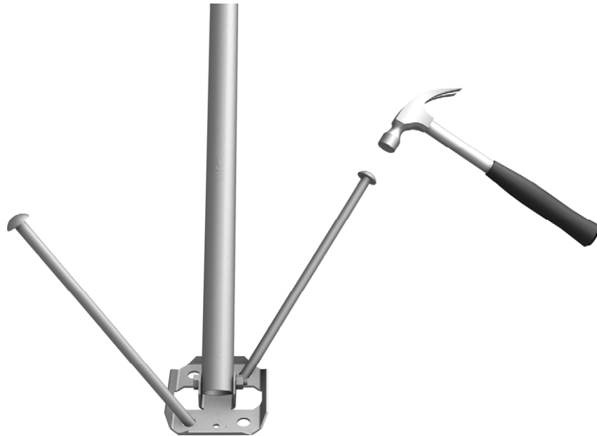
FIGURE 5-7. Staking the tripod feet
