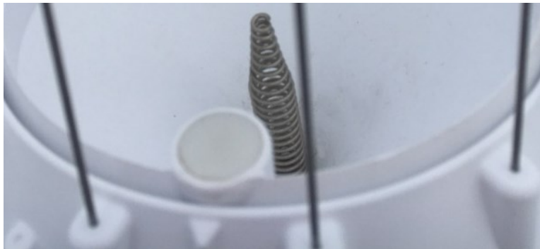
FIGURE 8-3. Correct installation: sensor is centered at the triangle
