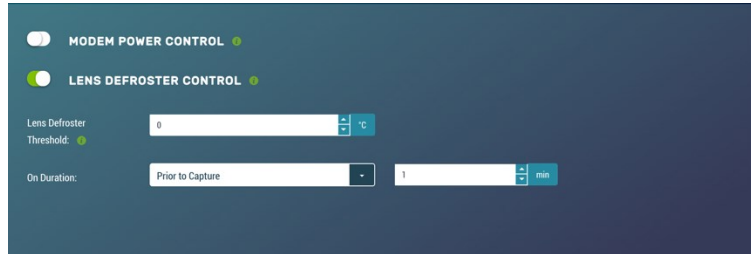
FIGURE 14-47. Lens Defroster Control: Prior to Capture
