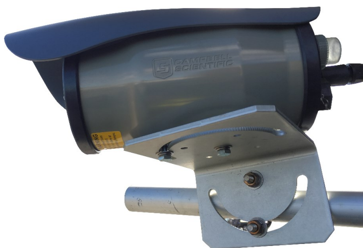
FIGURE 22-3. CCFC mounted to crossarm
