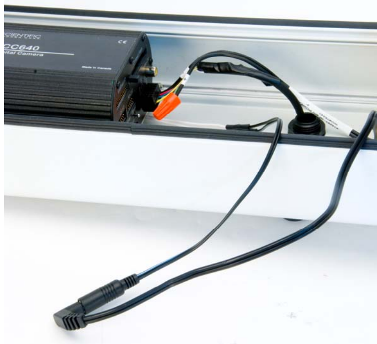
FIGURE B-4. Field Power Cable Connected to the Heater Connector
