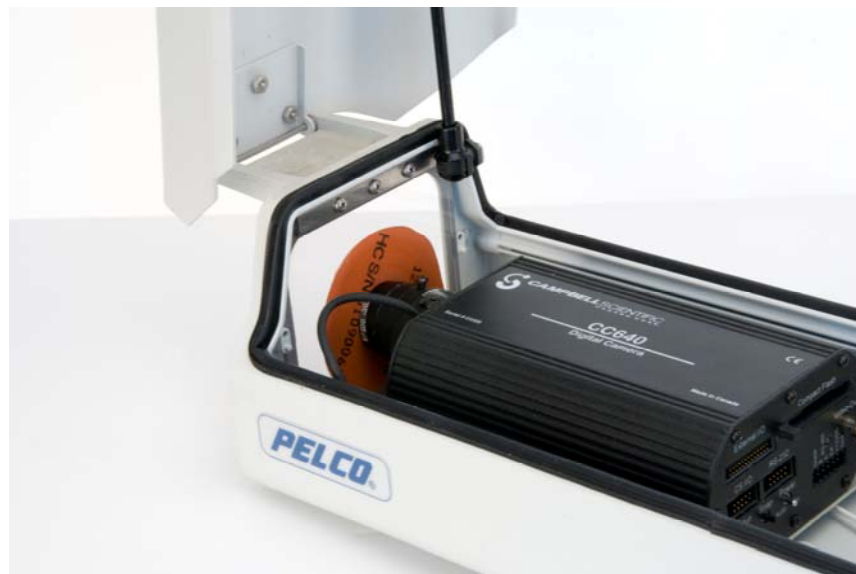
FIGURE B-2. Heater Properly Place in the Enclosure
