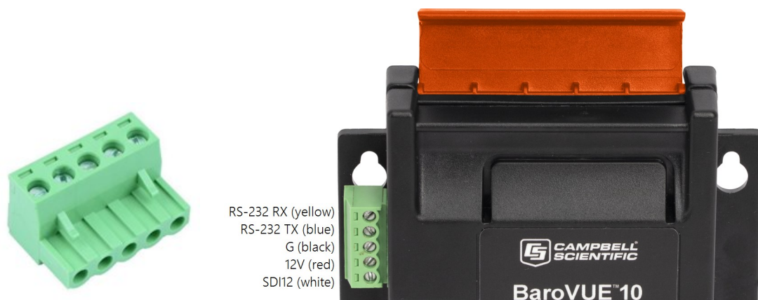
Figure 7-1. 5-pin screw terminal plug connector and connections
