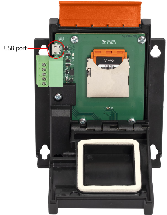
FIGURE 4-1. BaroVUE 10 with main door open
