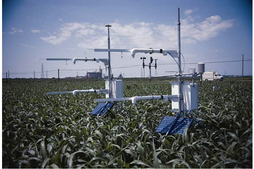
FIGURE 7-1. ASPTCs Mounted to Bowen Ratio Arms
