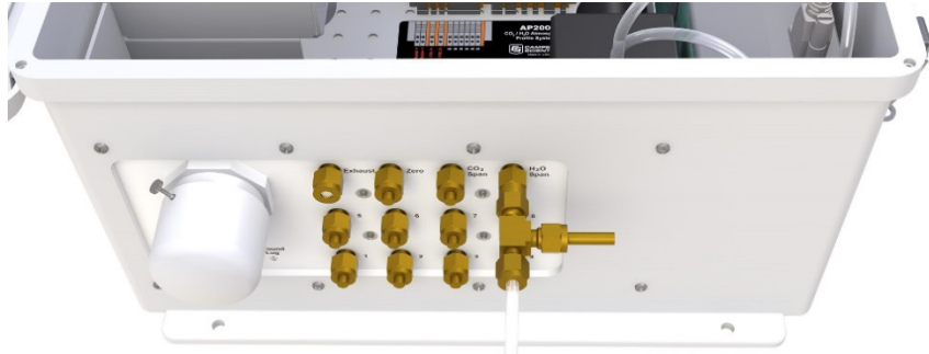
FIGURE 5-9. H 2 O span inlet configured for a dewpoint generator
