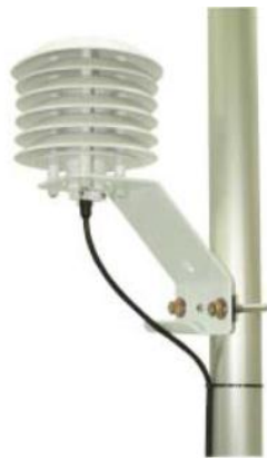
FIGURE E-1. 107-L temperature probe mounted with radiation shield
