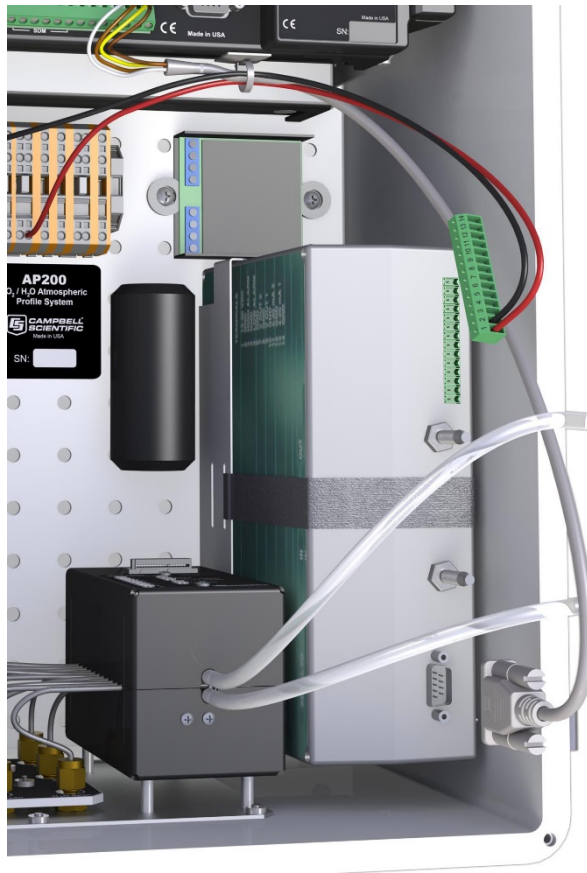
FIGURE 7-5. Components and fittings of IRGA installation
