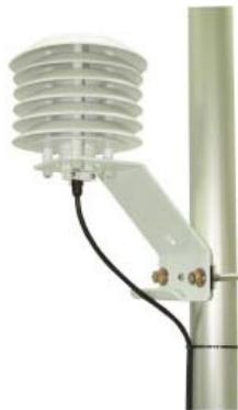
FIGURE 4-10. 107-L temperature probe mounted with radiation shield
