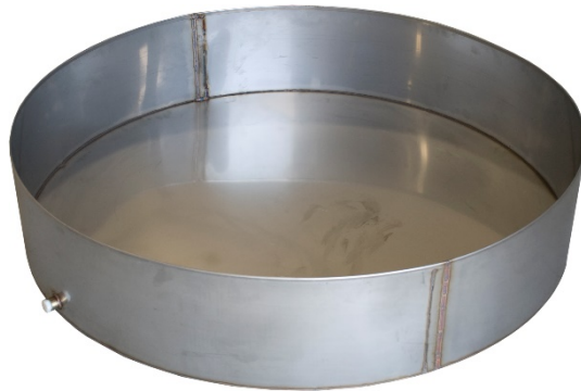
FIGURE 4-2. 255-200 Novalynx Class A Evaporation Pan
