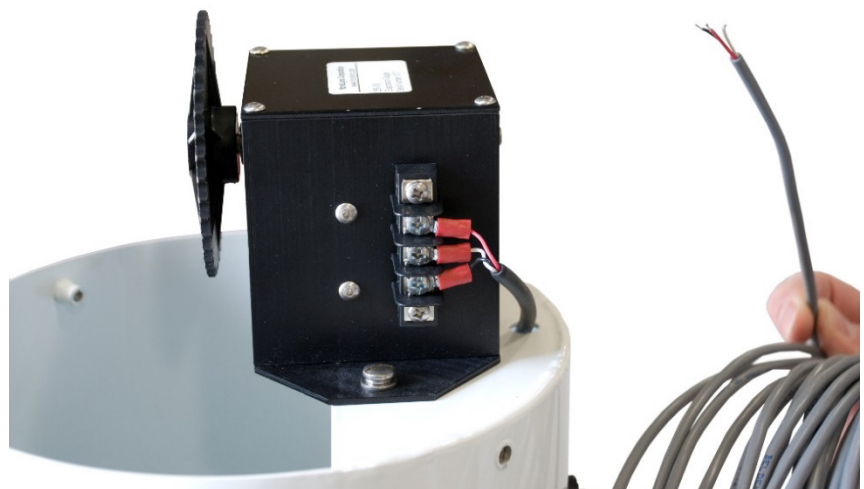
FIGURE 6-4. Close-up of Terminal Strip on 255-100
