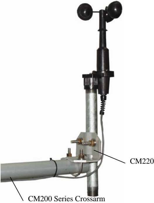
FIGURE 3-3. 03101 Anemometer Mounted to CM200 Series Crossarm with CM220
