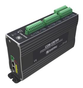
The CDM-VW305 is an 8-channel VSPECT vibrating wire module that allows high speed simultaneous vibrating wire measurements with traditional vibrating wire gages. Several CDM-VW305 modules can be connected to a single CR6 datalogger for a large channel count system; modules can be strategically located near sensors reducing cabling and installation costs without compromising measurement quality. Also available is a 2-channel model (CDM-VW300). U.S. Patent No. 8,671,758.
