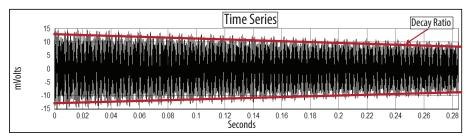
Traditional vibrating-wire readers determine the sensor frequency from the Time Series where signal and noise can't be distinguished.
