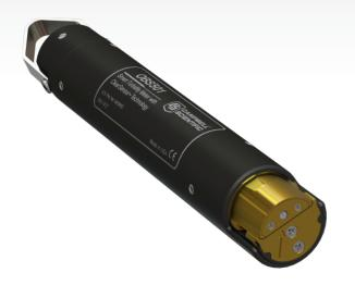
Turbidity sensors measure the amount of light that is scattered by the suspended solids in water. As the amount of total suspended solids (TSS) in water increases, the water's turbidity level (and cloudiness or haziness) increases. Turbidity sensors are used in river and stream gaging, wastewater and effluent measurements, control instrumentation for settling ponds, sediment transport research, and laboratory measurements.
