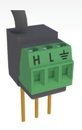
Resistive bridge adapters provide the completion resistors necessary for half-bridge measurements, help measure platinum resistive thermometers (PRTs), and are used with strain gages or other sensors that act as a single variable resistor.
