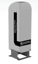
Campbell Scientific offers ceilometers that use lidar (light detection and ranging) technology to measure cloud height, vertical visibility, and mixing layer height. While they are best known for their use in aircraft operations at airports and oil platform helipads, ceilometers are also used by meteorologists for boundary layer research and air-quality applications.
