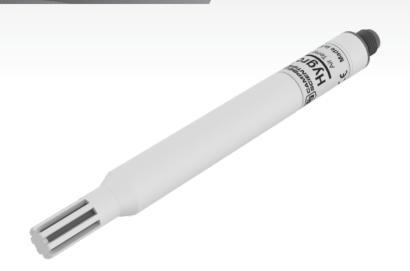
Air temperature and relative humidity sensors typically consist of two separate sensors packaged in the same housing. Often relative humidity is measured with a capacitive RH sensor, while air temperature is measured by a PRT.
