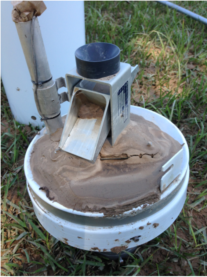
Sediment-filled rain gage
