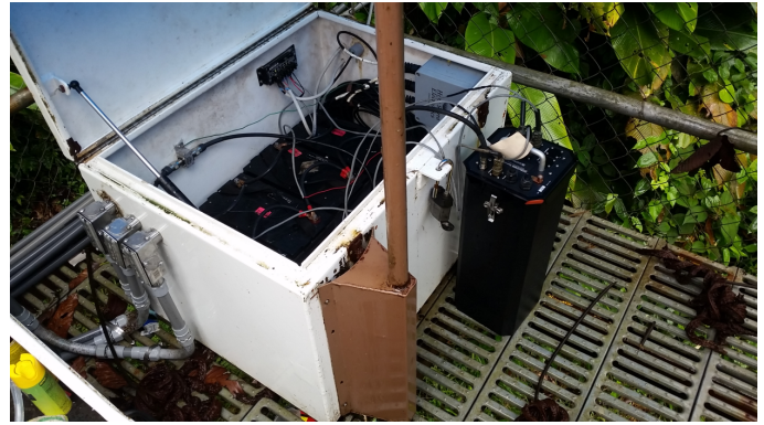
Campbell Scientific custom datalogger enclosure designed to meet WET specifications
