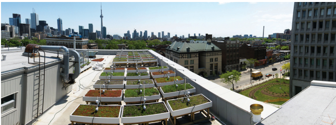
Automated weather stations monitoring 33 raised beds measuring 4 ft by 8 ft, with different soil media, amounts of soil, vegetation types, and irrigation regimes
