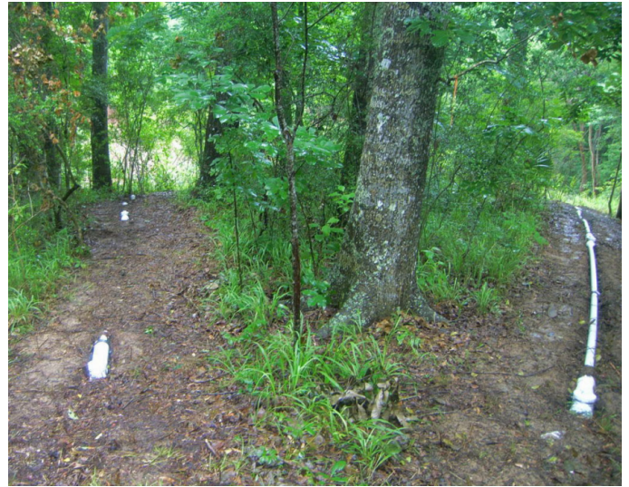
Two of the three arrays of telescoping PVC running from the data logger to the edge of the sinkhole
