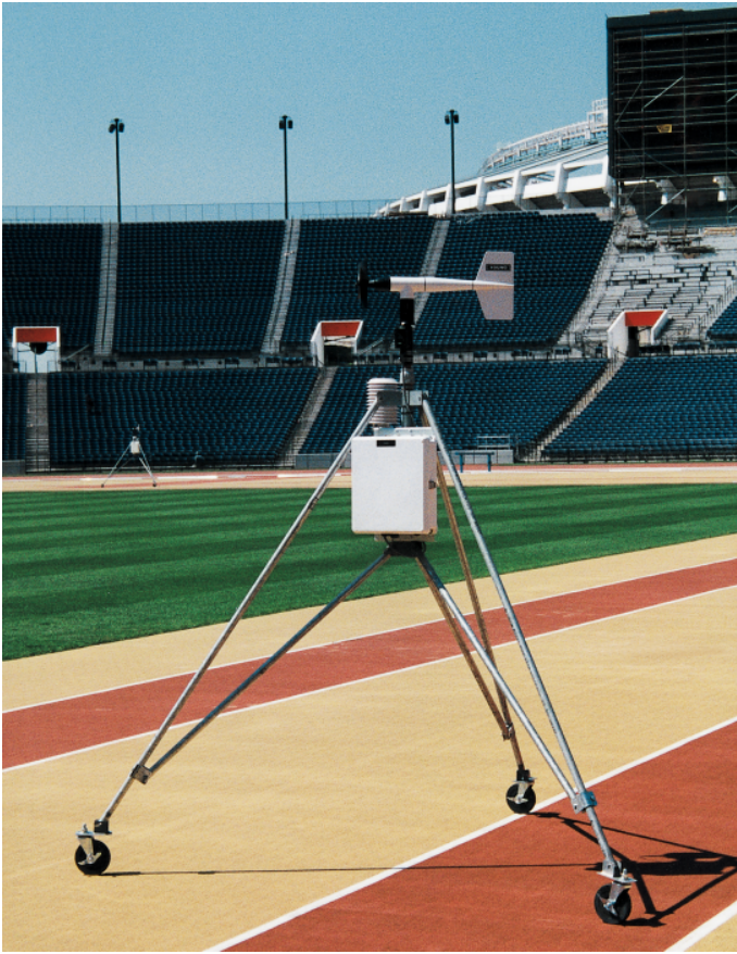
A mobile station was used to monitor meteorologic conditions at field level
