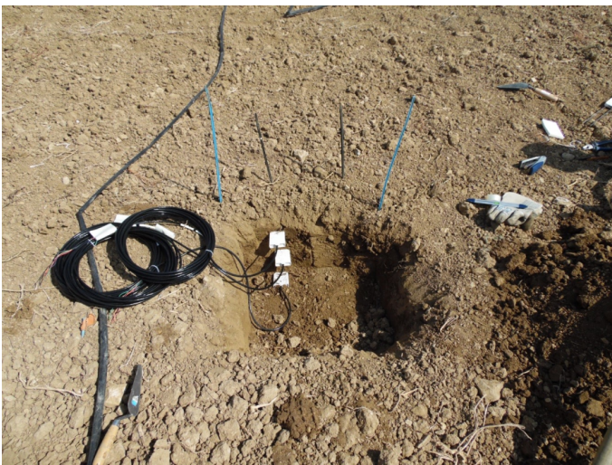
Monitoring of soil moisture volume and temperature (CS650 soil water content reflectometers)
