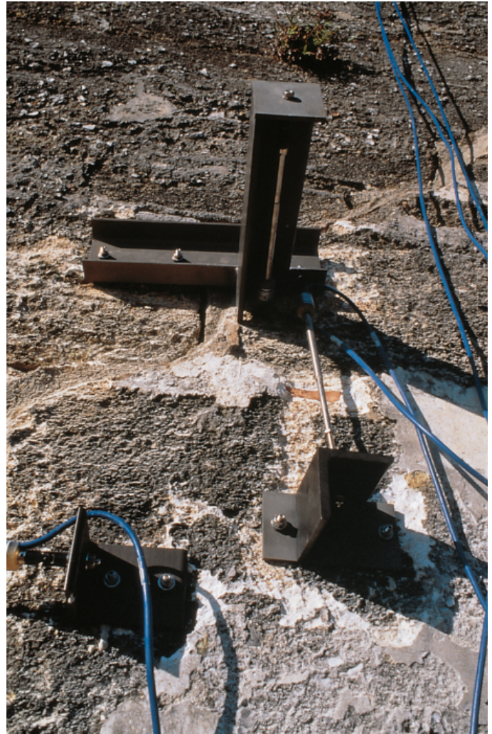
Sensors straddle cracks to directly measure displacement in each of three axes.
