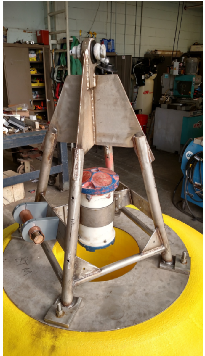
Buoy underside with an OBS501 Smart Turbidity Meter
