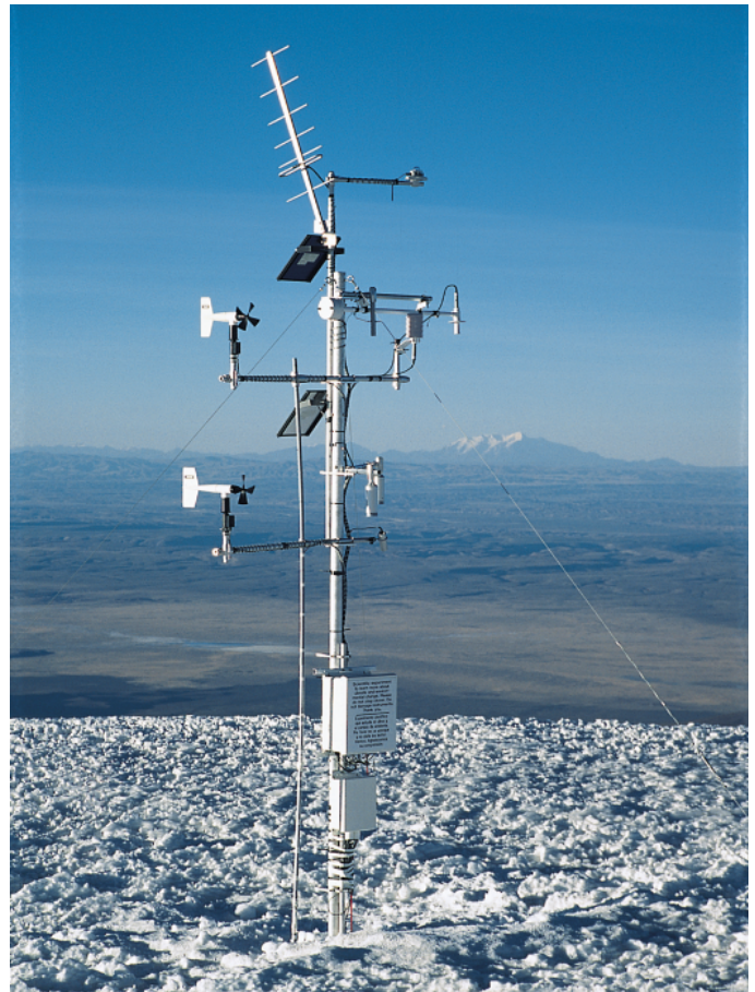
The Nevado Sajama weather station measures a variety of meteorological and snow parameters, many redundantly, to ensure data capture and integrity.
